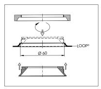
Now clip the PUNTEO®-J60 luminaire with the two lateral Clip springs into the upper part.
