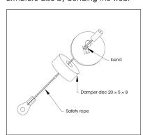
Then run the preassembled rope through an elongated hole [in the area of the later fastening points of the safety rope] in the rail channel out of the ceiling void downwards.  When assembling the LOOP® elements, the safety rope is screwed to the LOOP® element by means of a wing nut.
