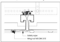
5. Measure the position of the LOOP® element exactly using the laser [longitudinal and transverse rows]. Hold the LOOP® element with the rear magnet [20 pieces per standard element] from below horizontally against the ceiling \$7 KS [friction force by magnet]. For the arrangement of the magnets, see below. To simplify assembly/disassembly, the magnets can be glued to the LOOP® element [e.g. LOCTITE].
