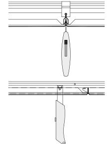
3. Pull the metal tile down until no more resistance is felt.
