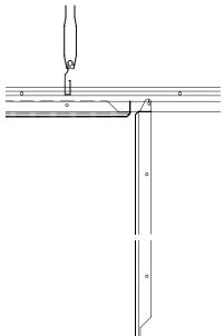
6. To remove the metal tile from the clipin carrier, the carrier must be spread open with a screwdriver.
